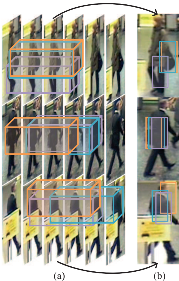
Fig. 8. 3D attentions of person samples in the iLIDS-VID dataset. (a) shows the recurrent 3D attention bins predicted by the proposed method in the original prediction video clips. To precisely visualize the locations of spatial attention regions, we draw the third frame of each video clip as examples and display the spatial regions in these frames in the part (b). Taking the first clip as the example, the part (a) of this figure shows that the learned attention bins focus on the frames with less occlusions from signboard, while the part (b) demonstrates that these attention bins focus on the salient spatial region (the bag). Best viewed in color.
